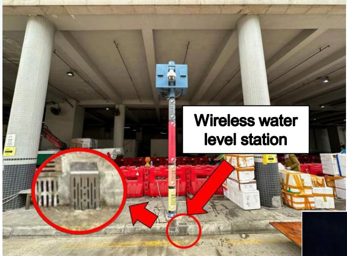
Therefore, we tested several **small wireless water level stations** near the existing stations. This gives us more **flexibility** in set up water level stations.
